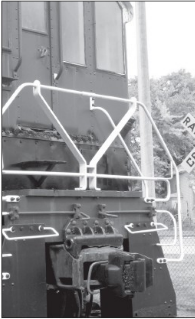
Damaged Rear Coupler on the 518
