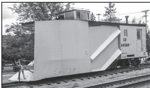
Conrail Russell double track snowplow #64568 with the lettering completed. It still needs new glass and floor work. (Carl Timko photo)
