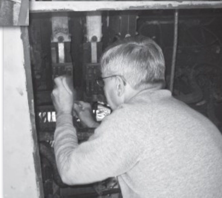
Prez Denny removes relays and contacts from Alco cab
