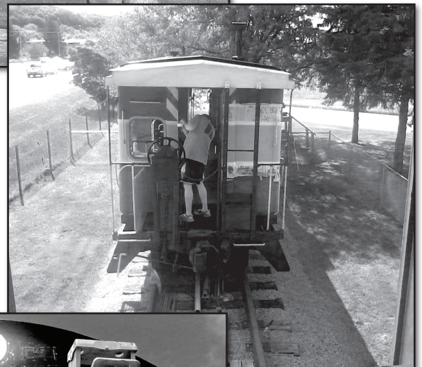
Masking of the caboose in preparation to touch up the gray band on the end of the caboose.
