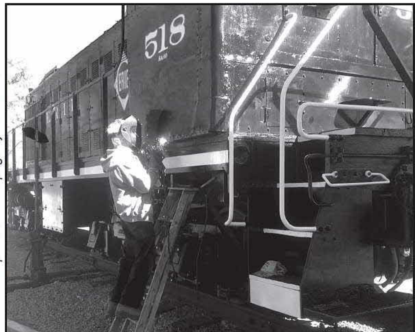
Stan Niwa welding a plate onto the cab of the 518.
