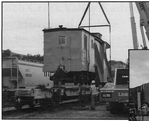
The Russell Snowplow being loaded onto a TTX owned flat car by Williamsport Crane at Wellsboro, PA - Dennis Mead photo
